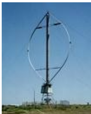
A Darrieus vertical axis wind generator. Also known as an "eggbeater".
